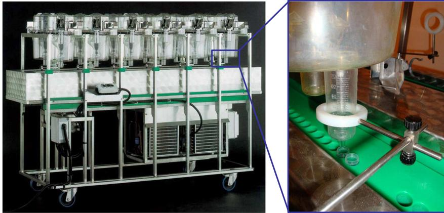
Figure 1: Overview of the refrigerated rack collector for 24-h urines collection
