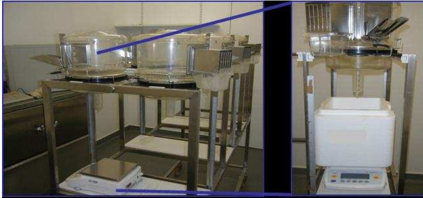
Figure 1: Metabolic cage with weighing device for spontaneous micturition evaluation
